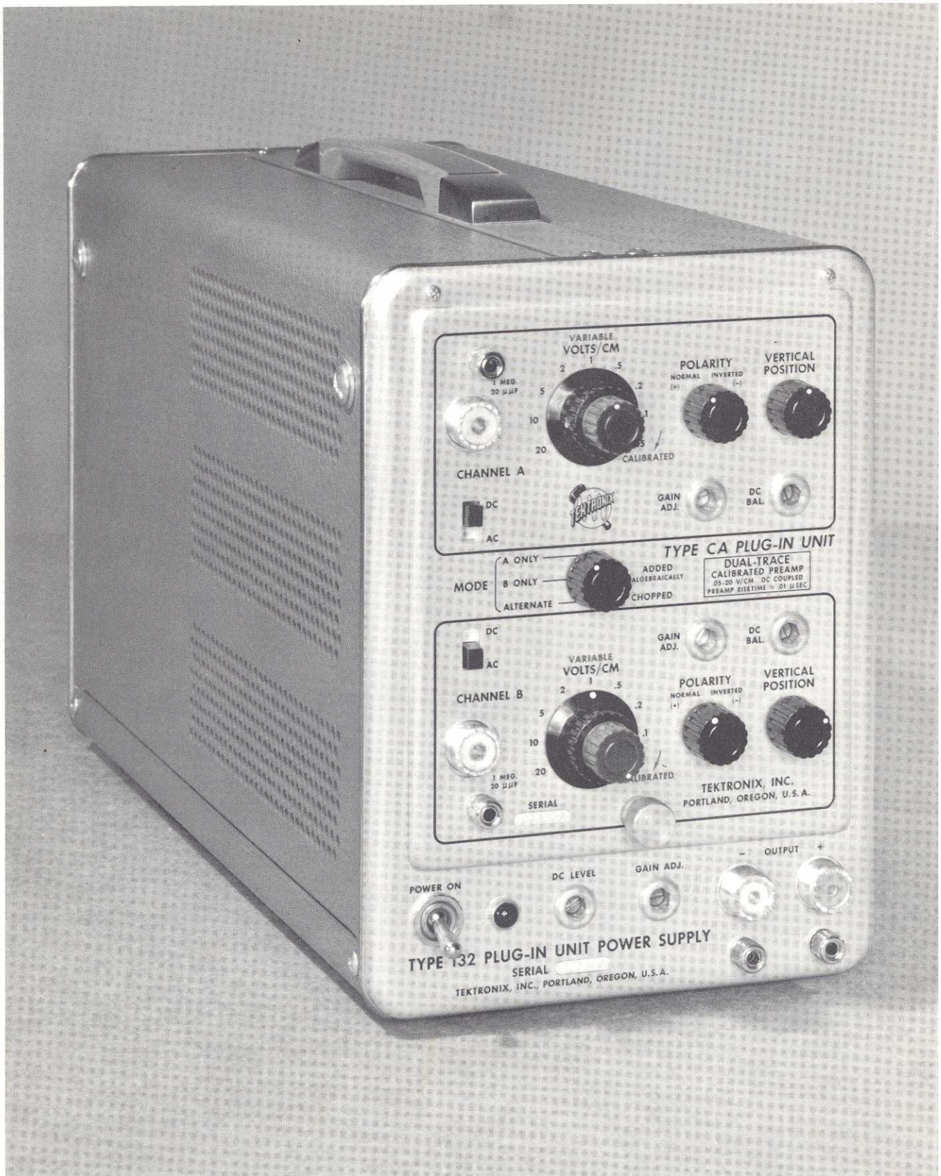
Fig. 1-1. The Tektronix Type 132 Plug-In Unit Power Supply with a Type CA Plug-In Unit.
